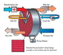
In the 1950's Munters invented modern industrial dehumidification when it introduced the selfregenerating desiccant rotor, the heart of the dehumidifier.
